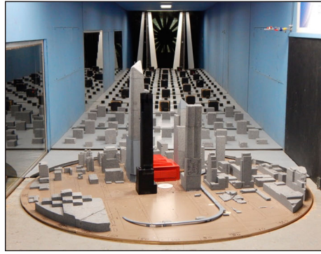
Fig. 13: Wind tunnel model for 35 HY showing the two configurations tested (© RWDI)
