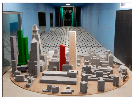
Fig. 11: Wind tunnel test models showing the three configurations tested for 1MW (© RWDI)
