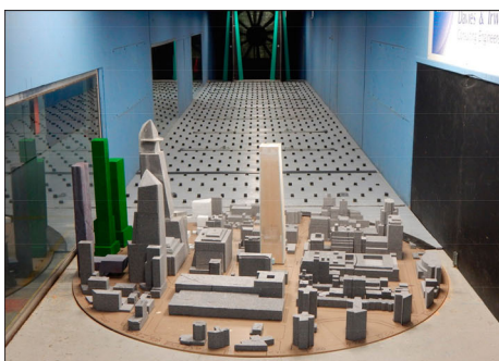
Fig. 11: Wind tunnel test models showing the three configurations tested for 1MW (© RWDI)
