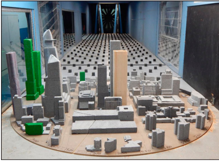
Fig. 12: Wind tunnel model for 2MW (© RWDI)
